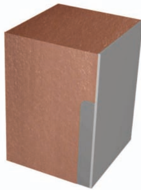
Nickel step-coating (variable thickness) with or without chromium layer
