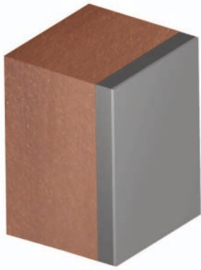
Nickel constant thickness coating with or without chromium layer
