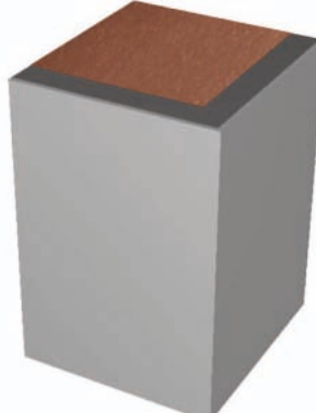
Nickel coating on edges with or without chromium layer
